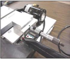
had only one inch of travel. This was overcome through the use of an aluminum block 1" X 2" x 3". Every time the micrometer reaches its limits, Tim retracts it and turns the block to the next largest dimension, and continues.
