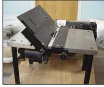
plate rip fence can be hit or miss, and stock has a tendency to want to "fall" towards the blade, which causes irregular cuts. Ray Oswald offered an excellent tip concerning the latter problem. Once you have the auxiliary table set to the correct angle, elevate one side of the table saw base; so the fixture is now on a level plane. This will help control the piece as it is fed through the saw.
